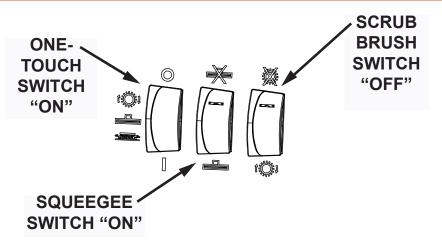
Fig. 1: Control Settings for Water Pick-up Mode
