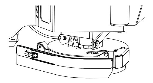
Fig. 1: Replacing the Side Scrub Brush
