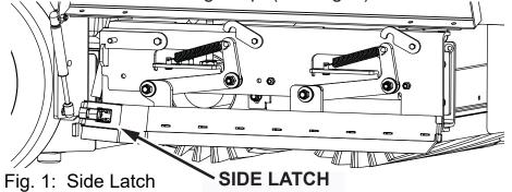
5. Replace the side squeegee blade by placing the blade onto the pins of the side squeegee frame.
