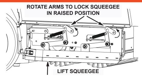
Fig. 1: Shows squeege assembly retaining arms
