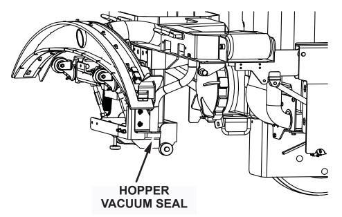
Fig. 3: Hopper Vacuum Seal location
