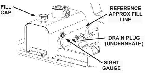
Fig. 1: Hydraulic Reservoir Nautilus Hi-Dump Rider Scrubber/Sweeper #988752UM Rev. A 07/16
