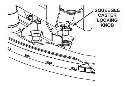
Fig. 1: Adjusting the Rear Squeegee Blade Flair
