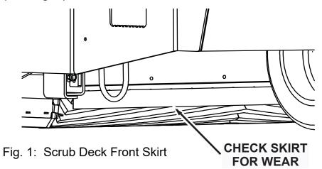
Check this skirt for wear or damage every 100 hours of operation.
