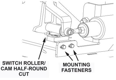
Fig. 2: Roller and Cam Position
