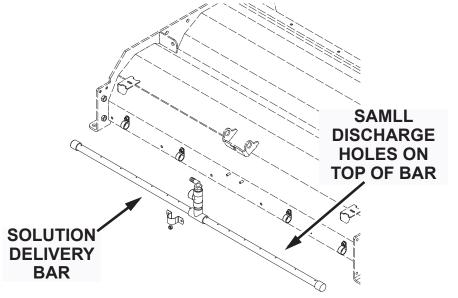
Fig. 1: Solution Delivery Bar shown with holes
