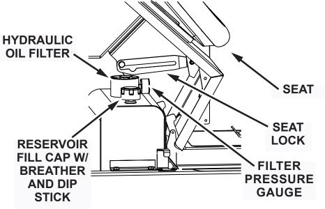
Fig. 2: Hydraulic Fluid Reservoir location
