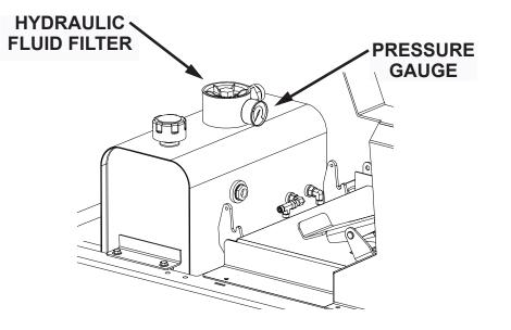
Fig. 2: Hydraulic Filter & Pressure Gauge
