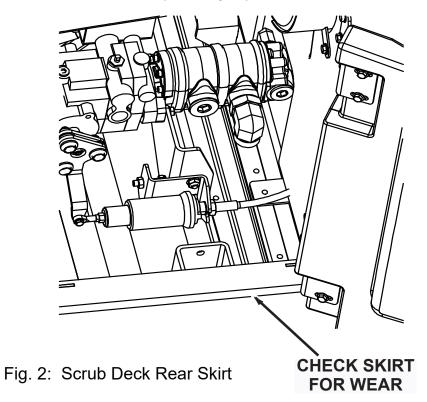
Check this skirt for wear or damage every 100 hours of operation.
