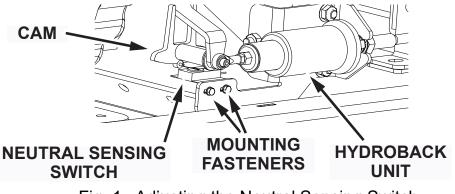
Fig. 1: Adjusting the Neutral Sensing Switch
