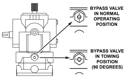
Fig. 2: Bypass Valve locations
