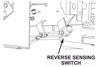
Fig. 3: Reverse Sensing Switch location
