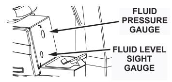
Fig. 3: Hydraulic Fluid Gauges
