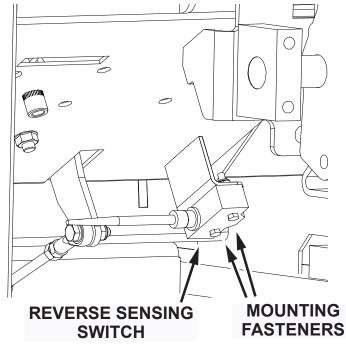
Fig. 1: Reverse Sensing Switch Fasteners
