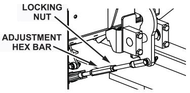
Fig. 2: Brake System Adjustment
