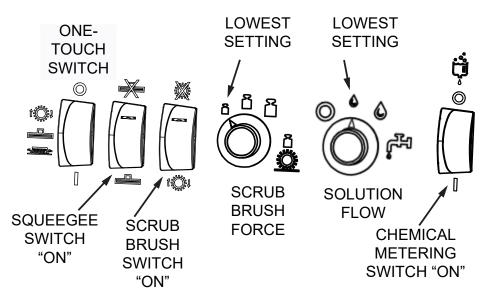
Fig. 2: Control Settings, before "One-Touch" selection
