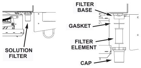
Fig. 2: Water Solution Filter with Exploded view
