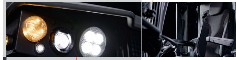
Brighter: Full LED lighting system with a high luminous efficacy and LED work lights for the brooms, the suction duct and the rear end of the cabin.
