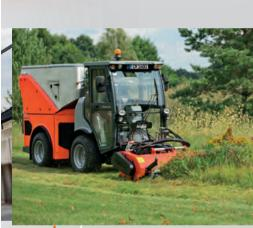
Mowing-suction combi unit with universal hopper: Mows lawns, maintains road-side greenery and works close to kerbs and edges on either side.
