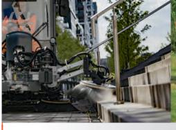
Can easily reach the next level: The additional broom provides simultaneous cleaning on different levels.
