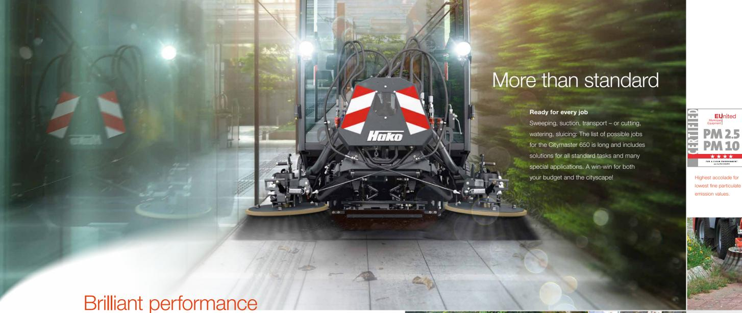
Sweeping is one of the main tasks in the field of Municipal Technology. The Citymaster 650 carries out all sweeping tasks rapidly, reliably and efficiently: thanks to its hydraulically driven 2-broom sweeping unit, quick-change suction duct and Intelli-Flap® coarse dirt flap. The machine's patented circulation water system provides maximum dust control – and ensures clean exhaust air and lowest possible dust and fine particulate emissions.
