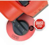
DustStop(option) reduces dust and fine particulate emissions at the side broom by up to 90 %.
