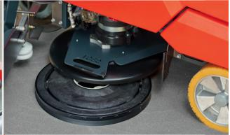
Rapid brush changing The automatic discharge and pick-up system provides rapid and comfortable changing of the brushes.
