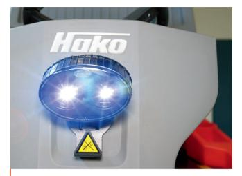
Increased safety in aisles The BlueSpot head lamp signals an oncoming vehicle.
