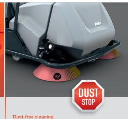
The optional pre-sweep/vacuum unit can be equipped with Dust Stop – our innovative disc brush jacket providing dust-free sweeping & vacuuming.
