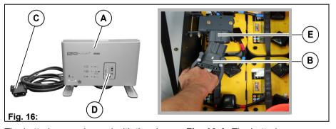
The batteries are charged with the charger **Fig. 16-A.** The batteries can already be charged when one segment in the charging status indicator **Fig. 14-51** has gone out.
