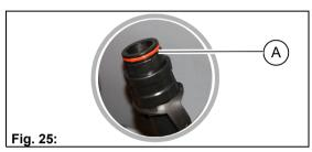
Check the function of the gasket at the drain hose **Fig. 25-A** daily, replace it after 125 operating hours at the latest.
